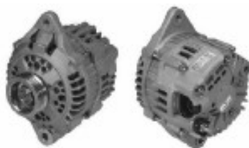
13713 LR190-737/737B/737E/737F NISSAN:23100-0W001/0W002 90A 12V CW 6S NISSAN PATHFINDER V6 3. 3L(1997-2000)
