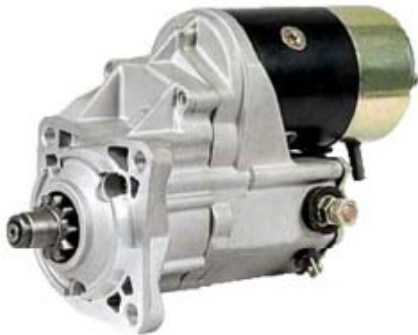
QDJ1206X1-000 12V/2.5KW/10T/CW LRS161
