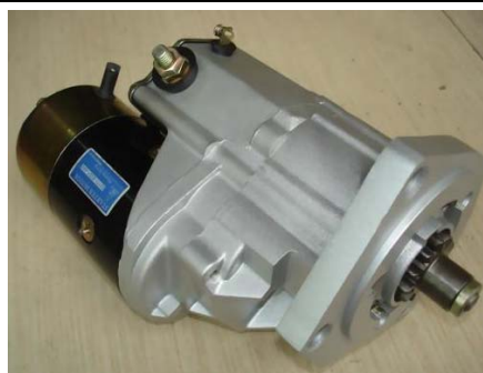
19748 24V/4.5KW/11T/CW 12V/2.5KW/11T/CW TOYOTA 13B 14B
